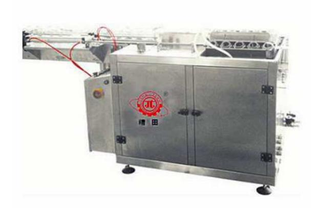
The machine uses the step/servo motor control roller intermittent rotary, high control accuracy, speed adjustment convenient. It uses the food grade pipeline design, attractive appearance, rational layout, simple structure, easy operation, steady production. By two water and five gas (Purified water, purify the heat) washing, drying, make the bottle meet the production requirements.
