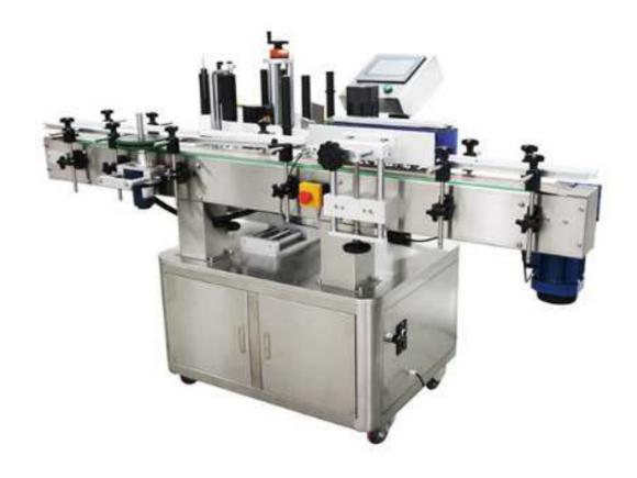
YTK-4 Full Automatic Labeling Machine is mainly composed of SS304 chassis; conveyor belt; Split bottle; Sponge wheel; labeling head; head adjustment etc. Use Siemens PLC, touch screen; servo motor as the main components, control devices run at high speed. Equipment safety, efficiency, and stability; comply with, CE specifications.
