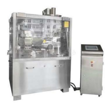
NJP-3500C automatic capsule filler processes the products for optimal productivity up to 3500 capsules per minutes, featuring low-maintenance operation, minimal downtime, and overall dependable production.
