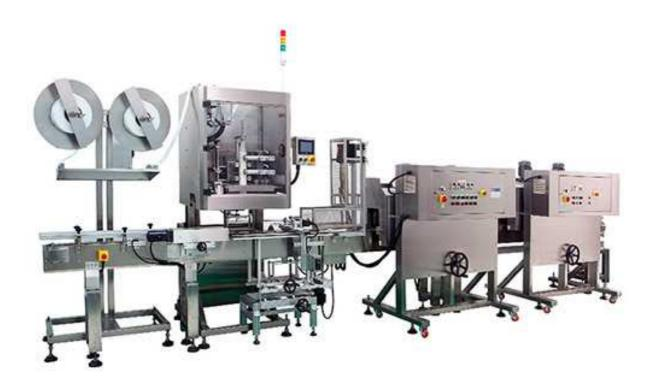
Auto Body Label Sleeve Applicator, LG-150 is designed matching CE certificate, higher safe standard. Machine is designed with SUS frame to match production requirement of Foods & Pharmaceutical industries.
