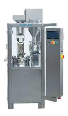
It is suitable for automatically completing capsule feeding, separating, filling, (waste capsule rejecting), closing, finished product ejecting for powder or tiny pill medicine in capsule. It is designed sophisticatedly by our factory according to the practice on domestic, It is fully accord with the GMP standard.
