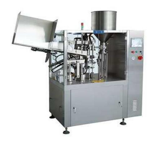
NF-60A Automatic tube filling & sealing machine adopts import foreign advanced technique, specially designed according to technology of cosmetics, ointment cream products, machine include automatic tube feeding, heating, sealing, pretreatment system, filling adopt mechanical piston, electrical control system and operation platform system.
