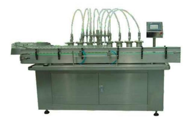
This linear filling machine is specially used for filling 50-500ml glass bottles and plastic bottles. 6-16 filling heads can be used, and its linear bottle feeding mode is very reliable. And there are no bubbles during filling process.
