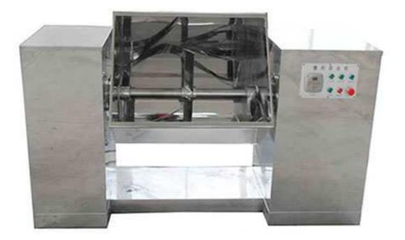
This machine is designed for mixing powders or pastes. It is a horizontal trough type mixer with single stirring arm. The stirring arm is removable so that it is easy to clean. The surfaces which may touch the mixing materials are all made of stainless steel 304/316L, so they have good corrosion resistance. The mixing trough can automatically reverse for discharging the mixture.
