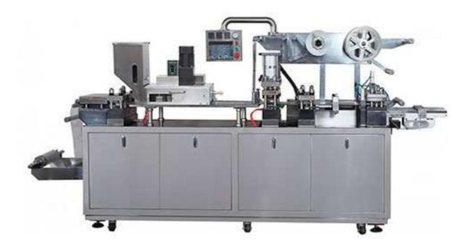
This machine is suitable for capsule, tablet, big honey pill, candy, liquid, paste, one injector as well as irregular shape Al-plastic and Al-Al sealing packaging in pharmacy, healthcare, food, cosmetics, medical equipment industry etc. This machine is adopted with micro-computer PLC, frequency converter, touch panel operation, high automation; it is ideal blister packaging equipment.
