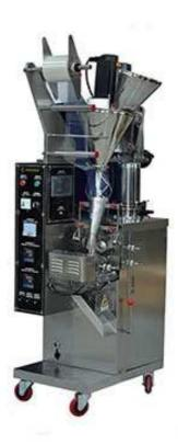
It is suitable for medical, food, chemical The machine used for packing a certain mobility, more loosely shaped, not all dust powder materials, such as flour, curry powder, lotus root starch, soybean powder, milk powder, strong bone powder, nutrition and food materials, continuous automated packaging.
