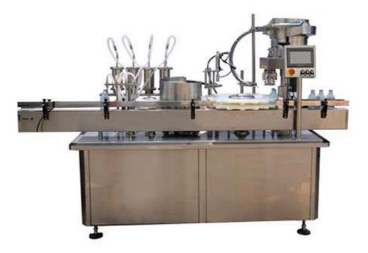
The machine is integrated with filling, inner plug, lock function. Mainly used for in-line production of large infusions and other small dose solutions, And can be equipped with a labeling machine to form a production line. The structure is compact, easy to maintain and simple operation, full compliance with the latest GMP requirements.
