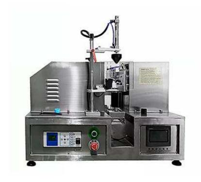
The working principle of the ultrasonic tail sealing machine is to vibrate through the high frequency of ultrasonic energy, and transmit the energy to the hose through the welding head. With the ultrasonic frequency of 20,000 times per second and a certain amplitude, the joint surface of the hose is violently rubbed Melting, communicating, and completing the gluing process in an instant, this process is called ultrasonic plastic welding.
