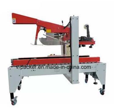
Automatic carton sealer is suitable for circumstance where the size of cartons does not change frequently, which especially fits for continuous sealing of cartons in the same size.
