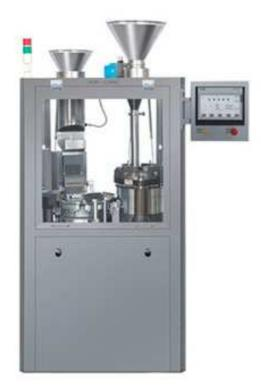
NJP-1200C Automatic Capsule Filling Machine adopts butterfly valve-type powder feeding, and is very suitable for drug powder with poor liquidity, including Chinese herbal medicine and Chinese patent drug, due to that its vibration unit equipped will force the powder to run down, which has solved problem of failing to feed in powder that often happens in the traditional screw feeding device because of the poor liquidity of powder.
