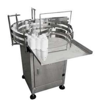
Bottle unscrambler is organizing different bottles to conveyors. It is widely used in widely areas, such as food, medicine, daily use, and chemistry. It is convenient to use and efficient, and easy to operate, meanwhile, have the high safety factors.
