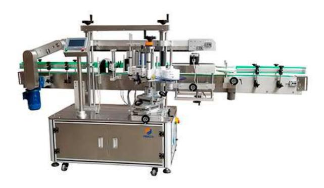
FK912 automatic single-side labeling machine is suitable for labeling or self-adhesive film on the upper surface of various items, such as books, folders, boxes, cartons and other single-side labeling, high-precision labeling, highlighting the excellent quality of products and improving Competitiveness. It is widely used in printing, stationery, food, daily chemical, electronics, medicine, and other industries.
