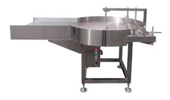
XJ-1000 Rotary bottle-feeding machine, adopts frequency converter changing the speed and rotary moving so that the bottles can standing orderly to the conveyor. It is the ideal replacement of the human labor. The equipment with compact structure can be applied to various sizes of bottle and without changing any spare part. It is an ideal equipment of the production line.
