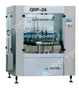
The machine mainly used for cleaning of glass bottles and PET bottles. It suits for full-automatic bottle cleaning before filling of wine and beverage manufacture, the capacity of the machine is about 3000-7000 bottles/hour. While it can be linked with filling line, it used continuous tracking way of cleaning, with high efficient, and perfect flushing effect, may be used in the different sizes of bottles and operation maintenance convenient.
