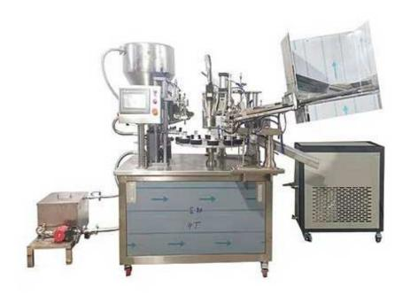
This machine is mainly used for quantitative filling and sealing of plastic composite hoses as packaging container materials. This machine is widely used in packaging in medicine, daily chemical, food, chemical and other industries.
