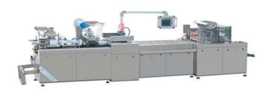
CD-5260 Battery Blister Packaging Machine is an ALL in one automatic card blister packaging system (Form/ Cut blister form/Product feed/Card supply/Seal) designed to meet a wide variety of packaging applications with high efficiency at economical price.
