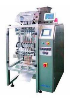
The high speed multi-filed bagging accomplishes bag forming, counting, filling, bag sealing and printing at the same time. Counts by infrared and sensor that doesn't wear or break the product and is compatible with all kinds of materials.
