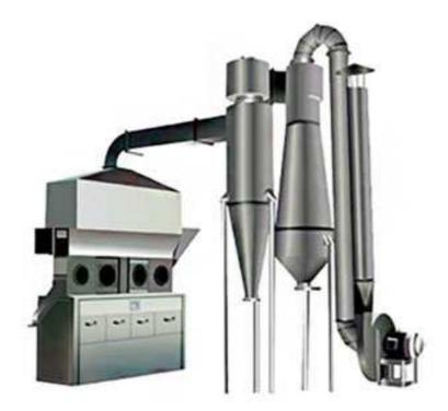
The clean and hot air enters into fluid bed through distributor of valve plate. The wet material is fed from the feeder forms the fluid state by hot air. Because of the wide contact between hot air and raw materials, the time of drying is short. If use continuous type, the material enters from the front of bed, fluidized in bed for several minutes, and float another side of bed. The machine works in negative pressure.
