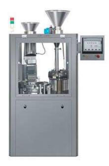
NJP 1200C automatic capsule filling machine can fill powder, particles and tablet materials into empty capsules. It can perform filling through stopples, batches and frequency control. The machine can conduct automatically filling, separating, (eliminating wasted contents) sealing up the powder or particle drugs to finished products.
