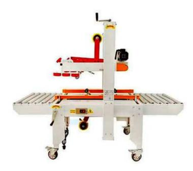
6060 drum type left and right drive carton packing machine adopts sticky tape to seal the carton, which is economical, fast and easy to adjust. It can complete the upper and lower sealing actions at one time, and can also use printing tape, which can improve the product image.
