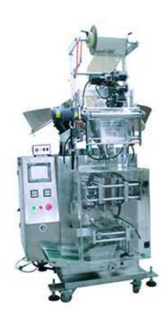
This series suitable for the full automatic packaging for round and ball material of foods, medicine, chemicals, such as sugar coated tablets, normal tablet, chocolate beans and capsule etc. This machine can pack 1-8 kinds tablets. We make the counting plate according to your tablets quantity.
