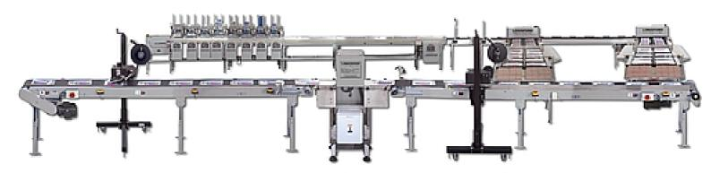
Provide system to decrease labour costs substantially & ensure proper collation sequence. Custom system that collates printed media, transfers to hand packing station for inspection into custom secure bags. Transfer onto flat belt conveyor for labelling and placement into packaging station. The system is approximately 1800 square feet.
