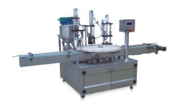
PLC control cylinder to make the piston reciprocate movement. The feeding valve will open when absorbing material. It will close when discharging, at the same time, opening filling valve to fill. User can adjust filling range, the material is not enough in the hopper, the computer will give the feeding pump signal to add material by level sensor. When the material is full, the pump will stop automatically.
