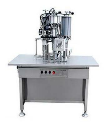
This machine is made from the former semi-automatic aerosol filling machine. It assembles the liquid filling, inflate and seal on the same table, it needs only one worker to operate it. It has high speed, high-accuracy and good stabilization and good choice and small-scale company.
