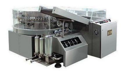
ACQ80 (60) (40) Ultrasonic wave washing machine is specially designed for automatic washing of various kinds of ampoules. This machine is mainly applicable for the washing of 1ml, 2ml, 5ml, 10ml and 20ml ampoules. This machine is of vertical rotation structure, it uses mechanic hand to clamp and overturn the bottle, it uses ultrasonic washing and water-air alternation spray to wash the bottle one by one.
