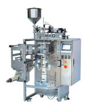
The main engine pump is made of stainless steel, the packaging volume can be steplessly adjusted within the rated range. Controller Chinese display, four-way sealing temperature controlling, reliable photoelectric detection system, automatically printing the batch number or production date, and the package finished cut easy to tear. Semi-fluid machine with mixing device can pack the sticky products with dregs, especially for instant food seasoning packaging.
