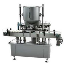
This machine is suitable for quantitative filling of different kind's granules. It adopts rotary type, air cylinder controls 12/18/24/32 discharge valves of filling valves and no-can-no-granules. The beating structure makes granules filling more easily. It is an ideal machine for rice porridge plants.
