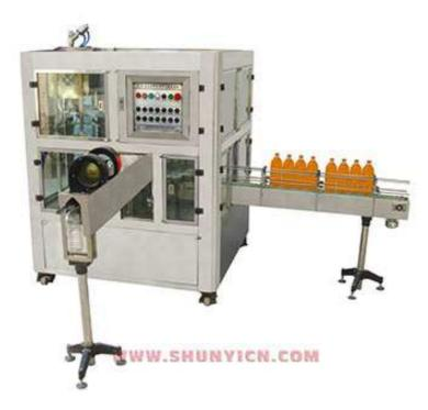
ZCX auto filling and capping machine is suite for fill and cap drink and milk with coconut, orange granular, pearl fruit etc
