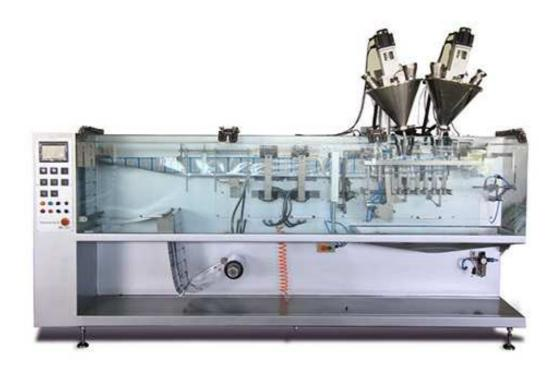
Pouch making, sealing and filling are relatively independent system. The two systems are connected by mechanical connection and PLC. Therefore, suitable for different packaging material and pouch sizes. Finished product sealing system uses hot seal packaging material to go on automatic pouch making, and so on. Pouches are doy pack, special shape, hanging hole. Selecting different filler can package different products.
