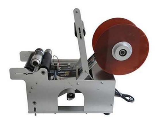
Semi automatic round bottle labeler is suitable for different size of adhesive film or adhesive label on all kinds of round bottle. High accuracy and high speed, dispensing & labeling automatically.
