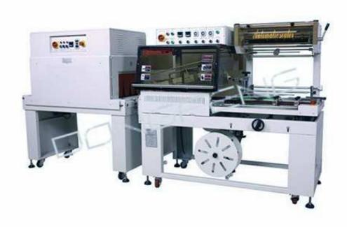
This automatic L-Bar Sealer Shrink Wrap Machine uses a belt to belt transfer system together with a synchronized film advance to transfer product from the in feed belt into the L-bar sealing area This automatic L- bar sealer is a production sealing machine capable of speeds up to 25 packages per minute - depending on package size and configuration of products.
