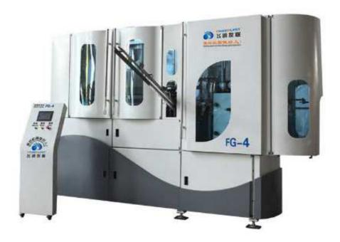
SMART series of blowing machine fills the gaps in field of domestic high-speed linear blowing machine currently. It has our own intellectual property rights, and has obtained more than 13 national patents. This machine is equipped with automatic perform loading and bottle unloading system. It is applicable for all shapes of drinking water bottles, carbonated bottles and hot filling bottles. FG4 is composed of three modules: preform elevator, preform unscrambler and host machine.
