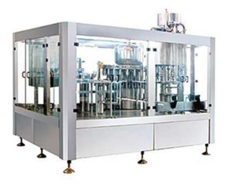
Washing, filling and capping machine is mainly applied for the filling of beverage. Integrating with washing, filling and sealing, it realizes full automation in the whole process, suitable for polyester bottle and plastic bottle filling of mineral water and purified water. The bottle types applicable for various parts are easily, conveniently and rapidly adjustable.
