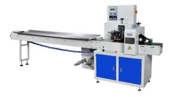
This pillow packing machine is designed to unitize product packs as well as to individually package piece products in three seal bags ("Flow Pack"). Suitable for non shape (irregular) products as well as normal product.
