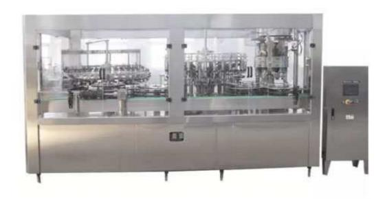
This glass bottle alcohol filling machine combines washer, filler, and capper (three-in-one monobloc) for wine (alcohol, spirit, liquor etc.)
