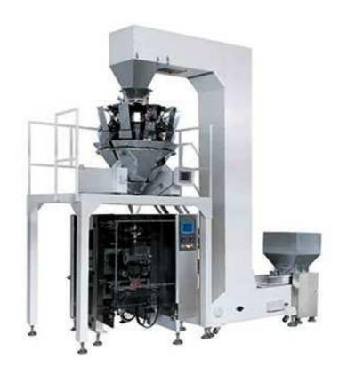
The Vertical Bag Granule Packing Machine is suitable for granule products like sweets, beans, peanuts, seeds, grain, biscuits, nuts, tea, dumplings, gourmet and ect.
