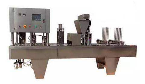
Linear Coffee Capsule Filling & Sealing Machine is automatic high-speed sealing machine. From drop cups, filling, put the film, print dates, twice sealing to out are all automatic operation. The electrical and pneumatic components are all using famous brands (can be also customized by customers' requirements), with stable quality, long life. It is mainly used in the products packing like: coffee powder, milk powder, rice, wheat powder and so on.
