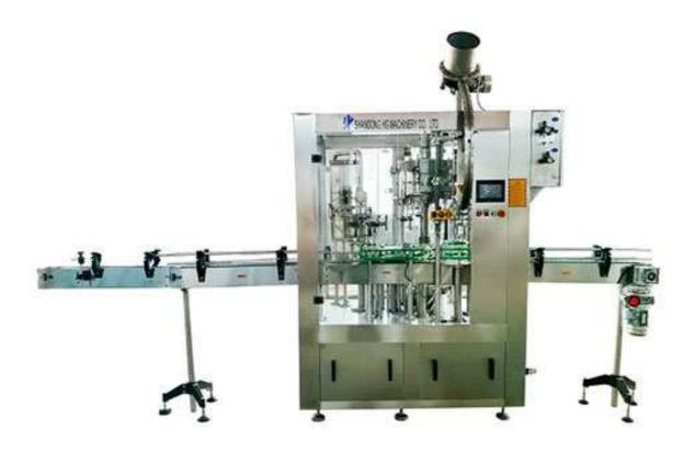
The 6 heads rinsing filling capping unit machine adopted European traditional filling valves, compact design small foot rint and low consumption, the ideal choice for small and medium capacity breweries the machine got three main parts: rinsing part, filling part and capping part. The machine filling use counter pressure filling method to ensure the beer good quality won't be influenced during the filling step
