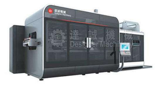
Our company is a professional thermoforming machine with tilting mold supplier in China. This kind of high automatic thermoforming machine adopts 15KW servo motor that offers high smooth and precision driving power. The max forming depth is 170mm and max working speed is 33molds.
