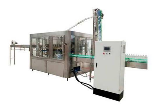
Automatic Sparkling Water Drinks Bottling Machine is mainly used for carbonated soft drinks filling, soda water drinks filling and sparkling water filling. It combines rinsing, filling and capping 3 functions. It suitable for PET or other plastic bottle. The iso-pressure (iso-barometric) filling technology is adopted enabling it to fill more efficiently and more stably with mor output than the machine of the same
