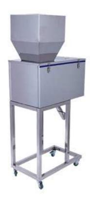
Fully automatic sub-packaging machine can be directly opened the pull button, remove the upper cover to clean the internal walkway, easy and convenient to remove. The product power cord is made of engineering plastic, high insulation, will avoid electric leakage, so that it is easy to run the machine
