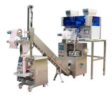
The triangle tea bag packing machine machine adopt the principle of ultra-sonic cutting and sealing, this will making the bag cutting is more evenly than traditional knife cutting and heat-sealing, for the ultra-sonic is more quiet running and tea bag sealing welding is more rigid, the tea bag is hardly crack and broken even soaked in 100 °C hot water. Besides the tea bag is with paper tag and cotton string, it is such convenient for consumer get out the tea bag and enjoy drinking.
