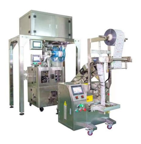
The tea packing machine is suitable for pyramid tea bag into an outer pouch package; it can make the inner bag into flat sachet or triangle bag and outer bag can be three side sealing bag; the complete line can automatic forming bag, weighing, filling, sealing, cutting, counting (optional), printing and output function.
