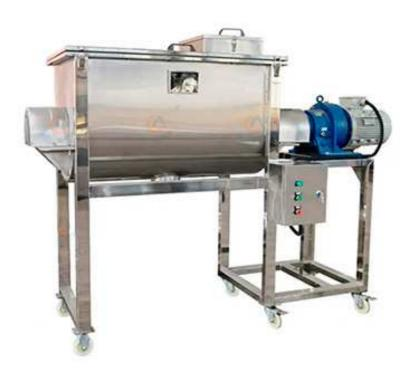
The milk powder ribbon mixer machine is designed to mix all kinds of dry powder. It consists of one U-shaped horizontal mixing tank and two groups of mixing ribbon: outer ribbon displace the power from the end to the center and inner ribbon move the powder from the center to the ends. This counter current action results in homogeneous mixing. The cover of the tank can be made as open in order to cleaning and change parts easily.
