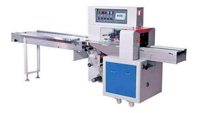
HU-350X under paper pillow type packaging machine is suitable for the packaging of soft objects, blocks, long strips and loose objects such as towels, paper towels, noodles, egg rolls, sausages, squid, popsicles, soft candy, biscuits and fresh fruits. Optional equipment has coder, straight line seal wheel, mesh end seal, large touch screen.
