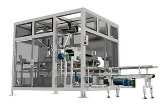
DCXLIA case packer is applicable to pouch bag auto packing production line which demands large capacity and high efficiency. It can complete the functions of material's auto arranging, auto positioning, auto gripping, auto packing and auto conveying out of case. It has the features of high-level automation, easy operation and steady performance.
